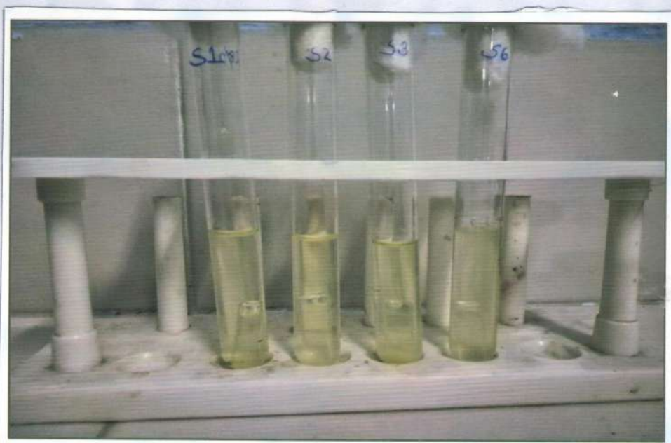
Lactose broth test result of Samples S1, S2, S3 and S6 shows acid and gas formation
