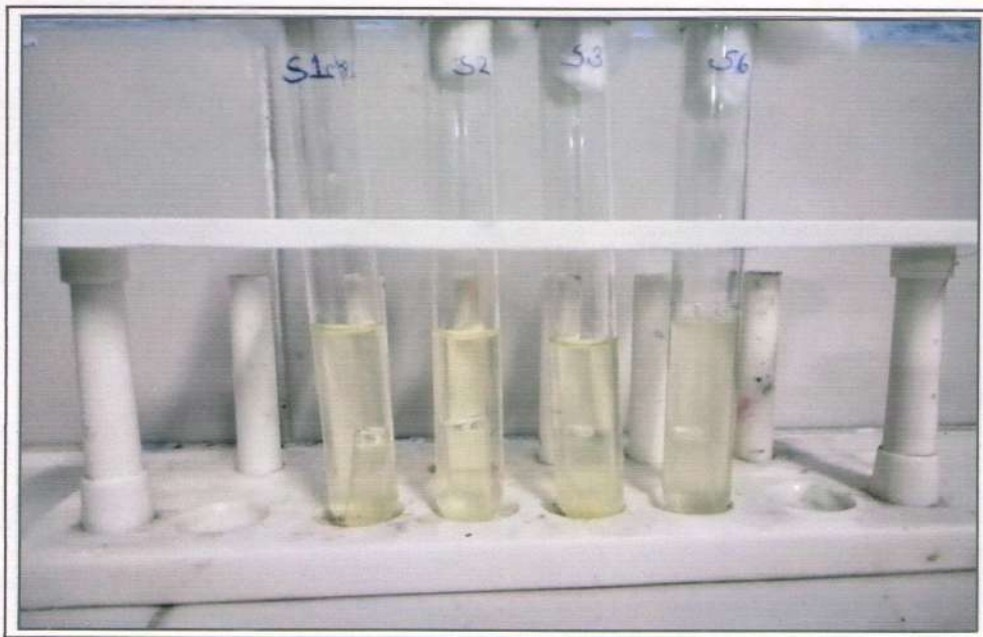
Lactose broth test result of Samples S1, S2, S3 and S6 shows acid and gas formation
