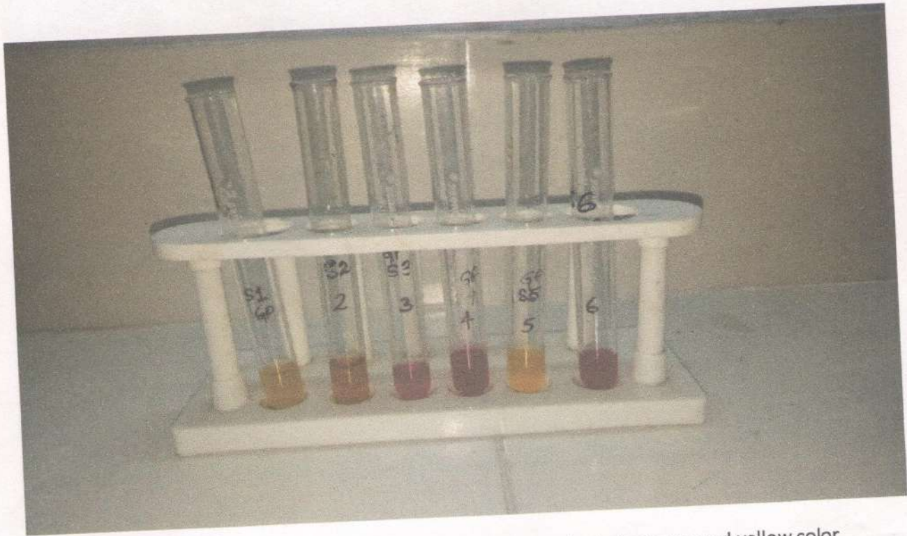
Methyl Red Test of water samples – S1, S2, S3, S4, S5, S6. Red colour indicate +ve and yellow color indicates –ve test.
