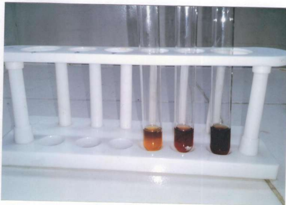
Fig 5: Methyl Test ! Red colour shows as positive, methyl test.
