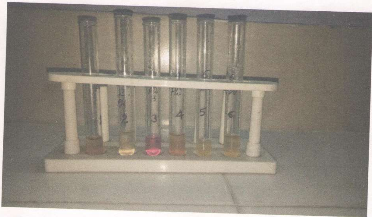
Indol Production Test of water samples – S1, S2, S3, S4, S5, S6. Red colour indicates +ve and yellow colour indicates –ve test.
