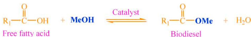
Fig. 2. Esterification reaction of FFAs using acid catalyst.
