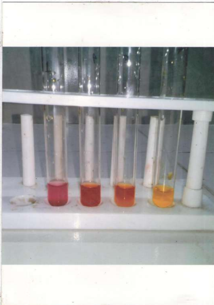
Fig 6: Production of red-pink colour which indicates the presence of indole in the samples.
