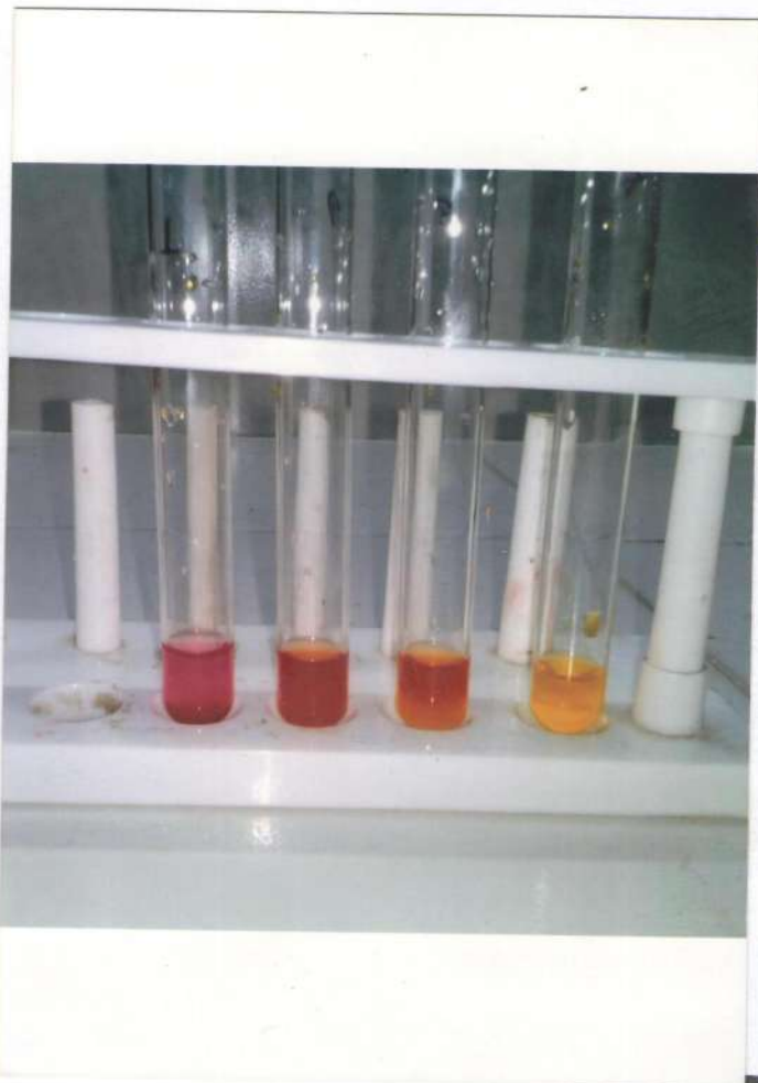
Fig:- Production of red pink colour which indicates the presence of indole in the sample.
